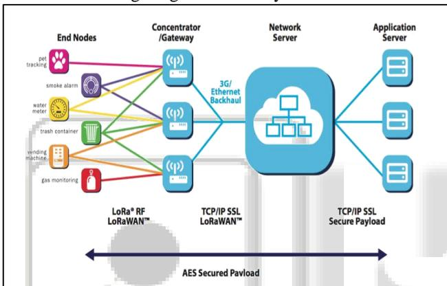
Fig. 4: explains the LoRa network which consists of several elements.
