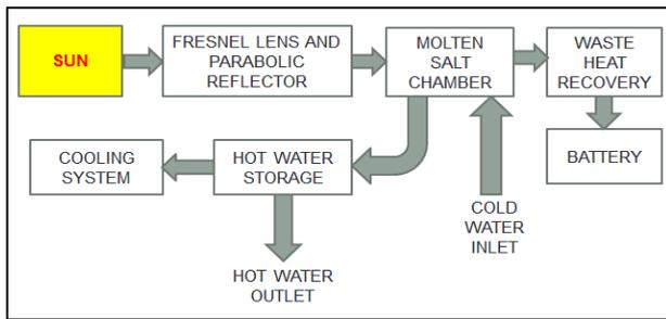
Fig. 1: Flow diagram
