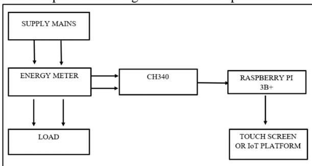
Figure 1: block diagram of the proposed system
