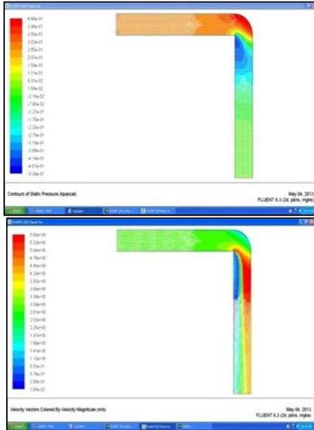
Fig. 9: CFD Analysis of fluid flow through 1” Elbow for 3m/sec velocity
