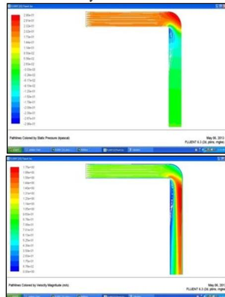
Fig. 3: CFD Analysis of fluid flow through  $\frac{1}{2}$ " Elbow for 1m/sec velocity
