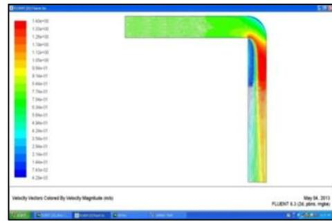
Fig. 6: CFD Analysis of fluid flow through 1” Elbow for 0.75m/sec velocity
