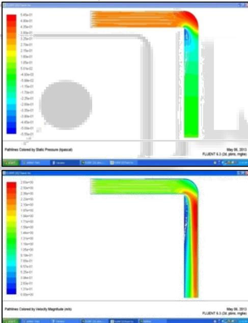
Fig. 5: CFD Analysis of fluid flow through ½” Elbow for 3m/sec velocity
