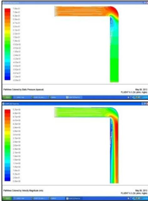
Fig. 4: CFD Analysis of fluid flow through ½” Elbow for 1.5m/sec velocity
