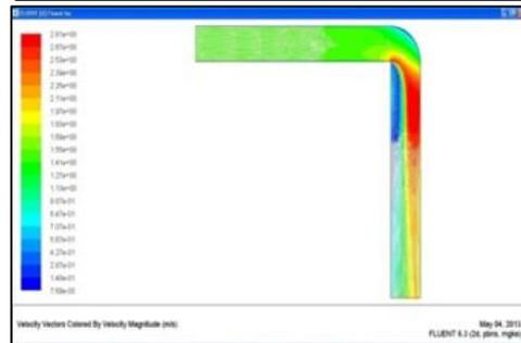
Fig. 8: CFD Analysis of fluid flow through 1” Elbow for 1.5m/sec velocity
