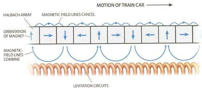
Fig.5. Concept of Inductrack
