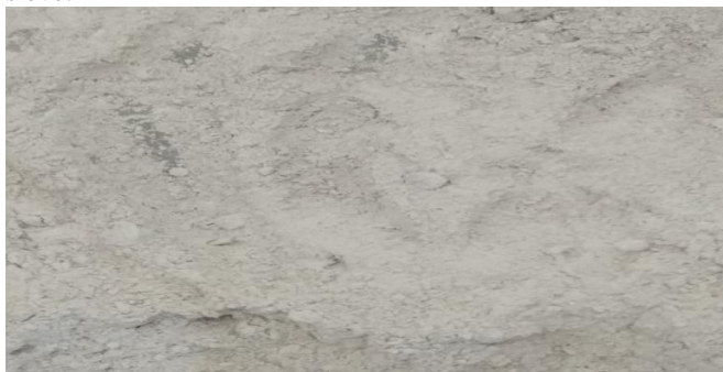
Fig. 2.1: Aggregate powder passed from I.S. 75 micron sieve.
