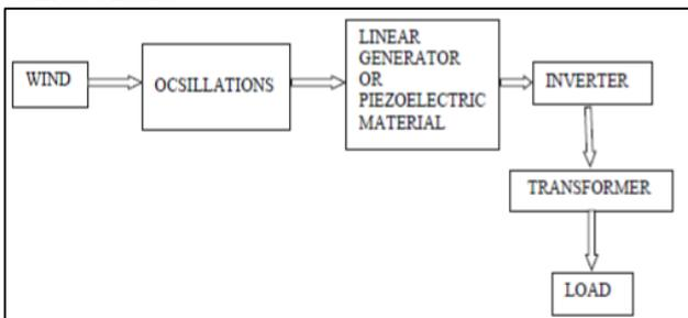
Fig. 2.2.1: Block Diagram of Bladeless windmill
