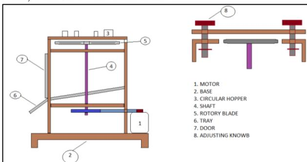
Fig. 1: Assembly of fruit slicing machine
