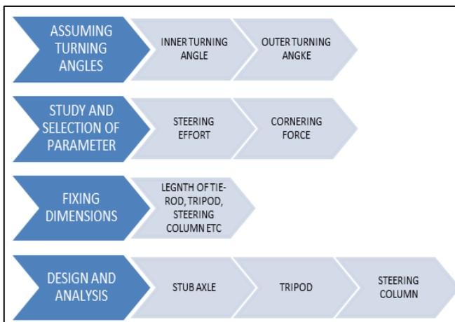
Fig. 1: Design methodology of steering system
