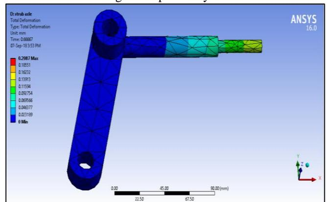
Fig. 4: Stub axle analysis
