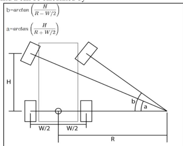
Fig. 2: constructional geometry of Ackerman
