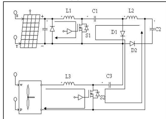
Fig. 3: Design of hybrid system when PV is available
