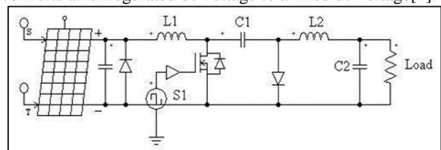
Fig. 1: Design of SEPIC converter
