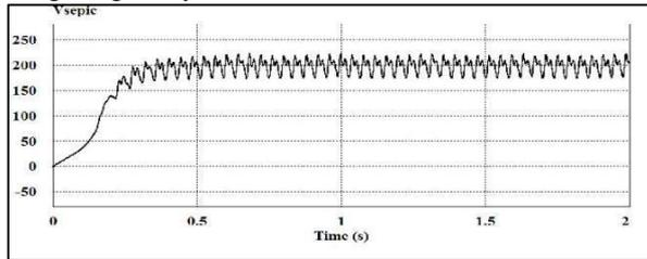
Fig. 2: Simulated output of SEPIC converter
