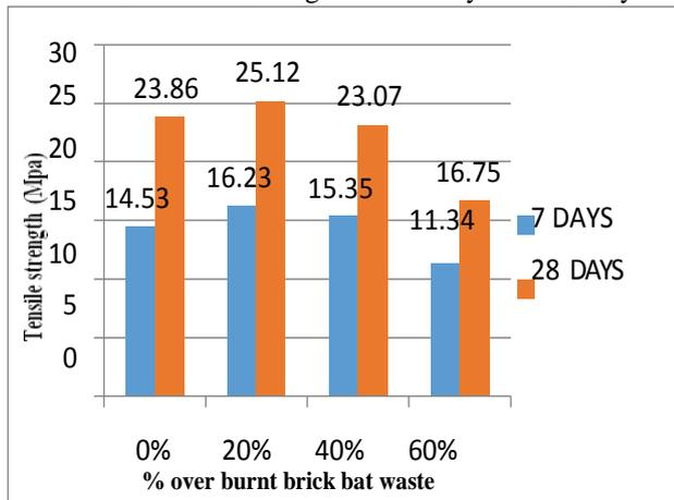
Fig. 3: Tensile strength after 7 days and 28 days
