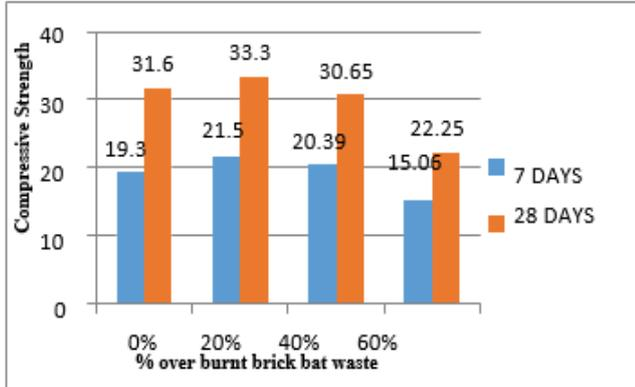
Fig. 2: Compressive strength after 7 days and 28 days
