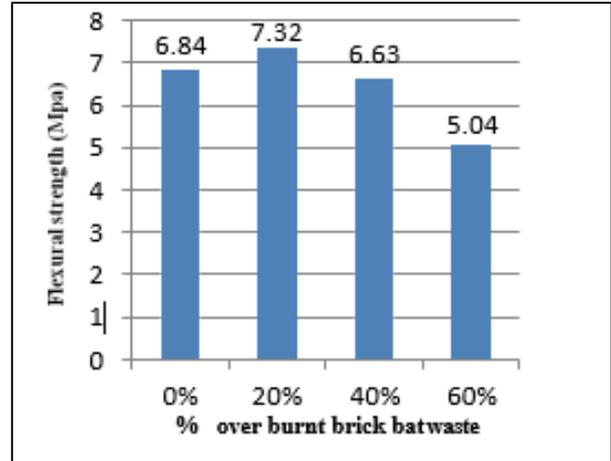
Fig. 4: Flexural strength for 28 days
