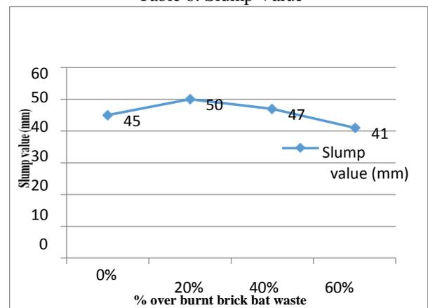
Fig. 1: Effect of over burnt brick on the workability of concrete
