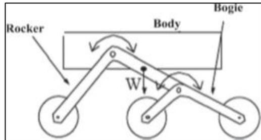
Fig. 2.1.2: Line diagram of Rocker-bogie suspension system.
