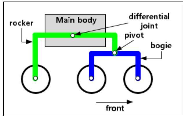
Fig. 3: Constructional dia. Of mechanism
