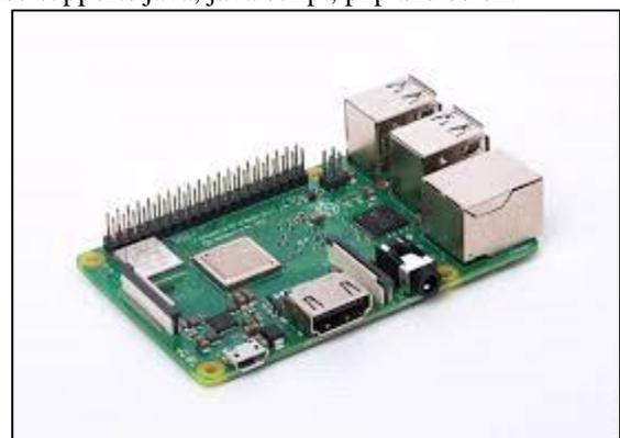
Fig. 1: Raspberry pi board
