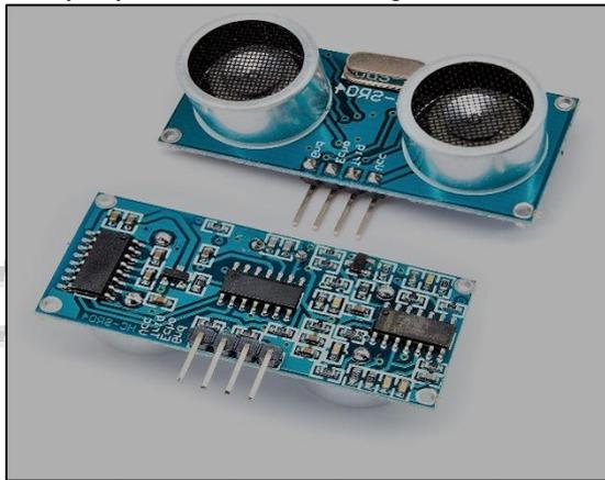
Fig. 2: Ultrasonic Sensor
