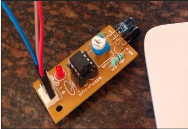
Fig. 7: Infrared sensor
