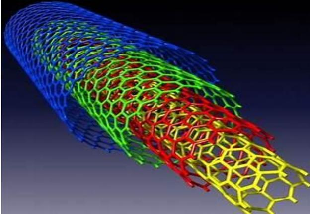
Fig. 7: Multi Walled Carbon Nano Tubes.
