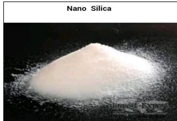
Is the first Nano product that replaced the micro silica. The Nano silica powder is one of the blended material. Studies have shown the existence of silica powder, in the early cement hydration product Ca (OH) 2 content along with the growth of the age becoming less and less, even complete reacted, generate new material which will jam channel, big pores will less, cohesion between aggregate and plaster will be strengthen, compactness will be improved.
