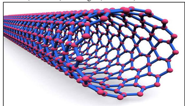
Fig. 6: Single Walled Carbon Nano Tube
