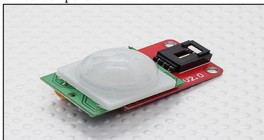
Fig. 4: Body Movement Sensor
