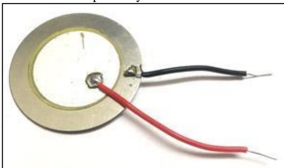
Fig. 3: piezoelectric sensor
