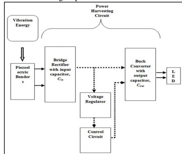
Fig. 4: block diagram of architecture
