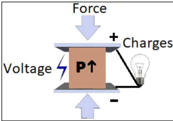
Fig. 2: diagrammatic representation of piezoelectric sensor
