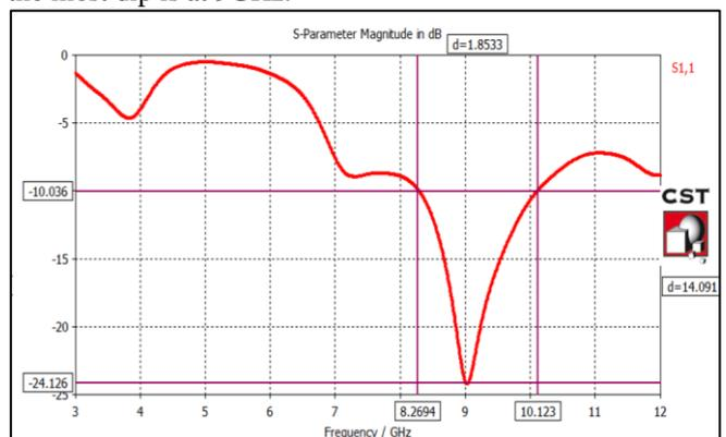
Fig. 3: S-parameter, S11 in dB
