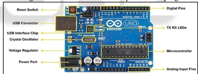
Fig. 1.3: Arduino pin diagram
