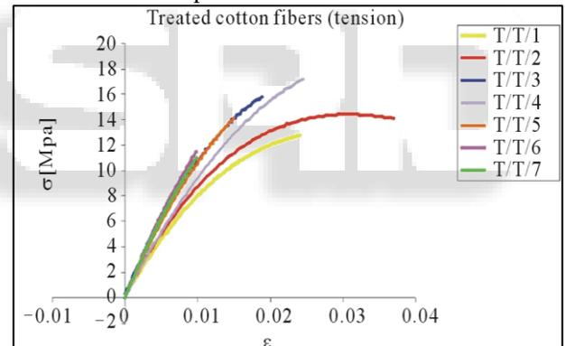
Fig. 6: Stress-strain curves for treated cotton fiber specimens in tension.
