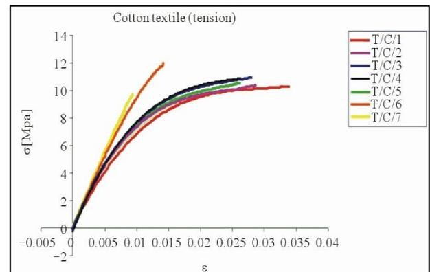
Fig. 7: Stress-strain curves for cotton textile specimens in tension.
