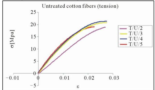
Fig. 5: Stress-strain curves for untreated cotton fiber specimens in tension.
