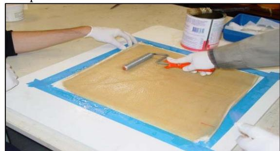
Fig. 2: Plate specimen preparation.
