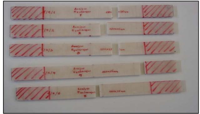
Fig. 4: Failure mode of plate coupons in tension.
