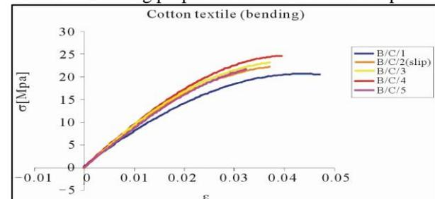
Fig. 10: Stress-strain curves for textile cotton specimens in 3-point bending.
