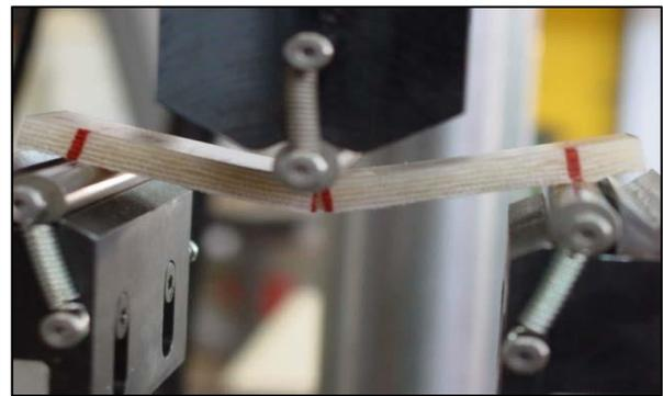
Fig. 8: Failure of coupons in 3-point bending.
