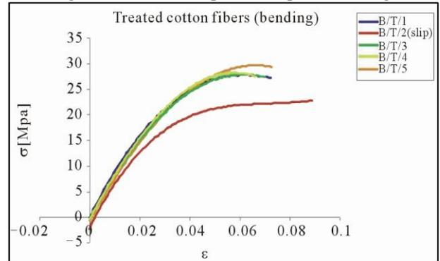
Fig. 9: Stress-strain curves for treated cotton fiber specimens in 3-point bending.
