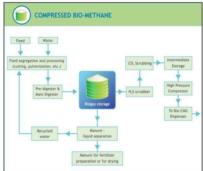
Fig. 2: Diagrammatic Representation of Compressed Bio-Methane Production
