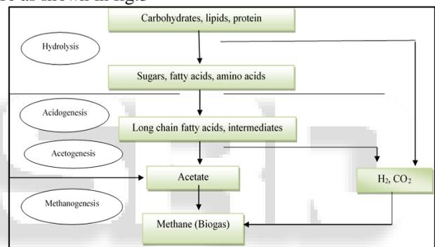
Fig. 3: Chemistry of Anaerobic digestion
