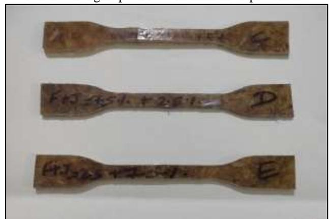
Fig. 2: Tensile test specimen
