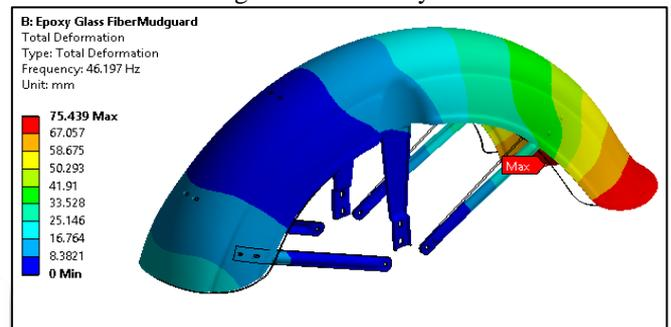
Fig. 5: Results of Composite Mudguard
