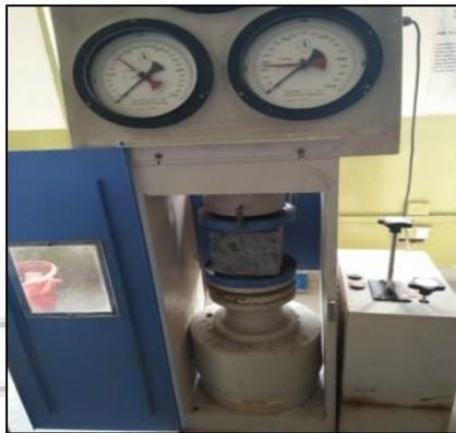
Fig. 3: Compressive strength of cube
