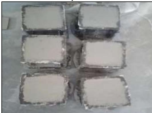
Fig. 4: concrete cubes casted in the mould
