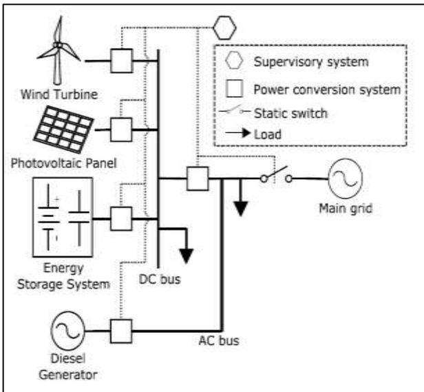
A. Architecture of a Microgrid
