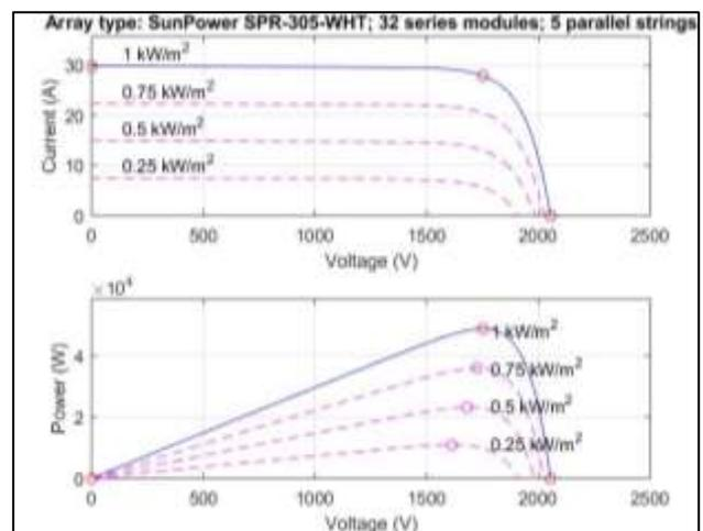
I-V and P-V characteristic of PV array
