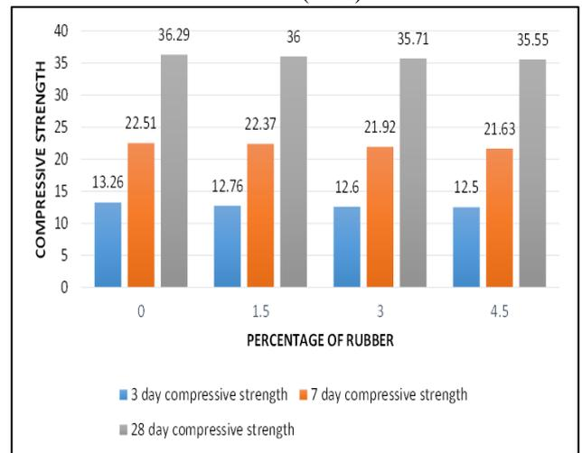
Fig. 6: 3, 7 and 28 days Compressive Strength for different percentages (by total volume) of rubber at 1.5 % human hair content (M30).
