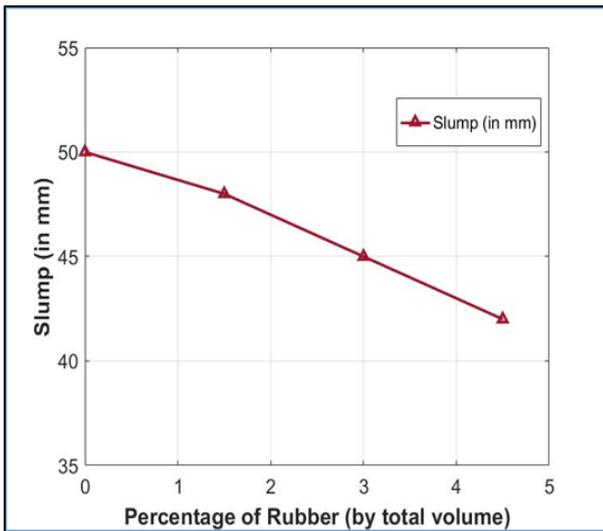
Fig. 2: Slump values for different percentages (by total volume) of rubber and 1.5 % human hair content (by weight of cement)
