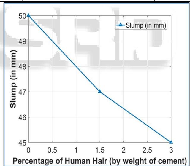
Fig. 1: Slump for different percentages (by weight) of Human Hair
