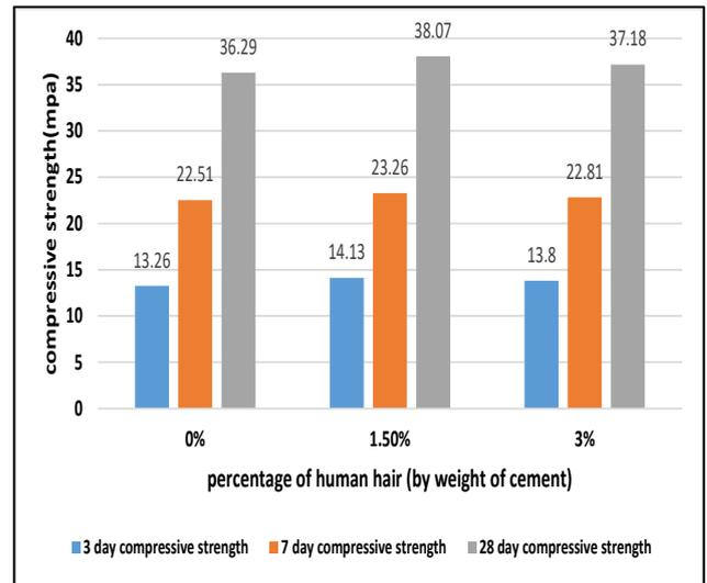
Fig. 4: 3, 7 and 28 days Compressive Strength for different percentages (by weight) of Human Hair
