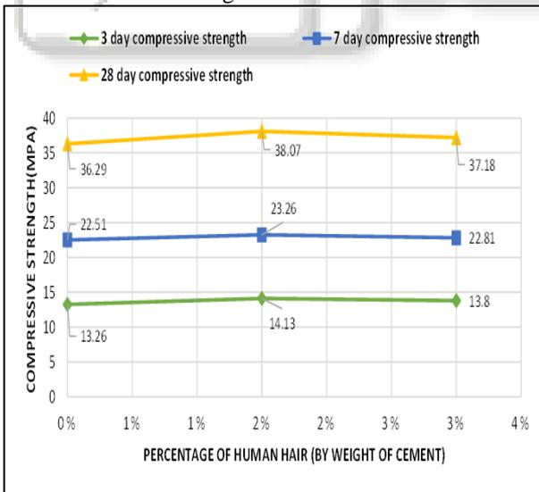
Fig. 3: 3,7 and 28 days Compressive Strength for different percentages (by weight) of Human Hair.
