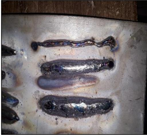
In this parameters arc gap is too short and too long and the results are in this photo.
