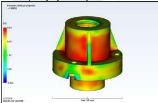
Fig. 2: Optimum Volumetric shrinkage at ejection
