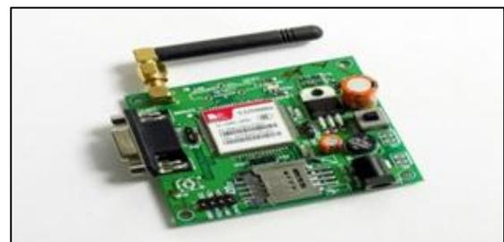
Fig. 4: GSM Modem
