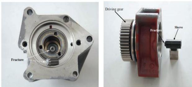
Fig. 4: Failed auxiliary driving assemble. Yu et al. 2012
