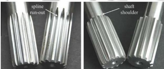
Fig. 8: Spline shaft design with spline run-out or shaft shoulder Shen and Lohregel 2013
