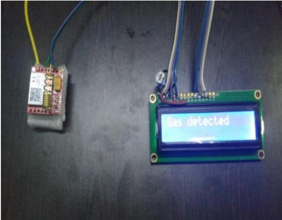
Fig. 2: Display of Gas Detection on LCD
