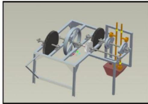
Fig. 3: Basic Components in Chilly Crusher Machine
