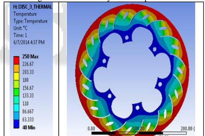
Fig. 3.32: Thermal Analysis of sample disc 4
