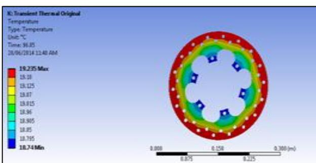
Fig. 6.1: Transient Thermal Analysis Result- Selected Disc (sample disc 1)
