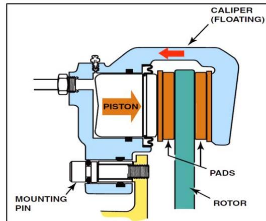
Fig. 1.1: single-piston floating caliper disc brakes
