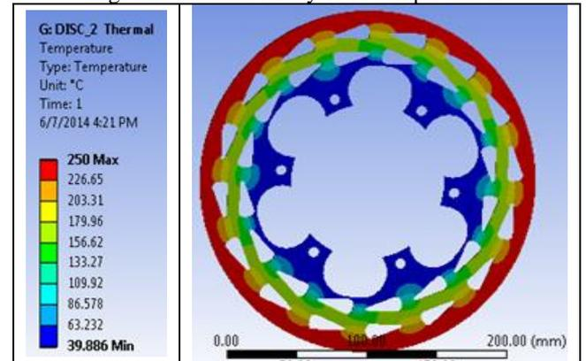
Fig. 4.3: Thermal Analysis of sample disc 3
