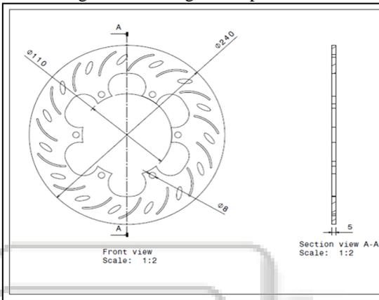
Fig. 3.4: Drafting of sample disc 4
