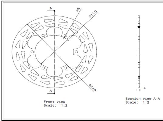
Fig. 3.3: Drafting of sample disc 3
