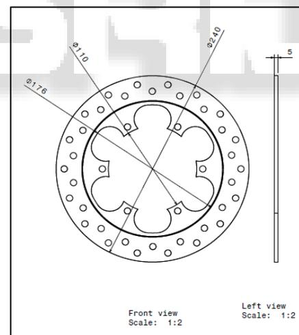
Fig. 3.1: Drafting of sample disc 1
