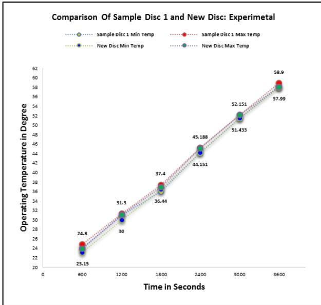
Fig. 8.1: Comparison of Sample Disc 1 and New Disc: Experimental
