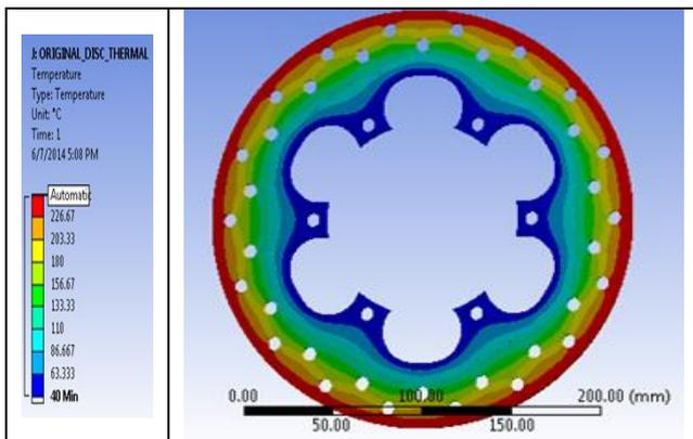
Fig. 4.1: Thermal Analysis of sample disc 1
