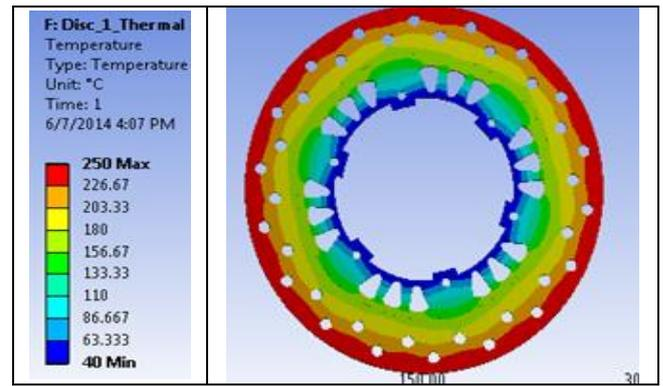
Fig. 4.2: Thermal Analysis of sample disc 2
