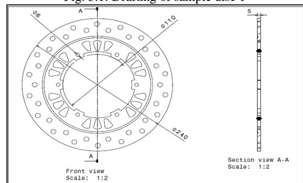
Fig. 3.2: Drafting of sample disc 2
