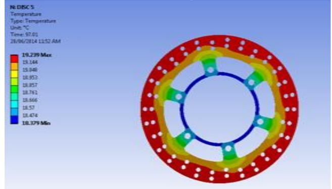
Fig. 6.2: Transient Thermal Analysis Result (ANSYS) of New Disc
