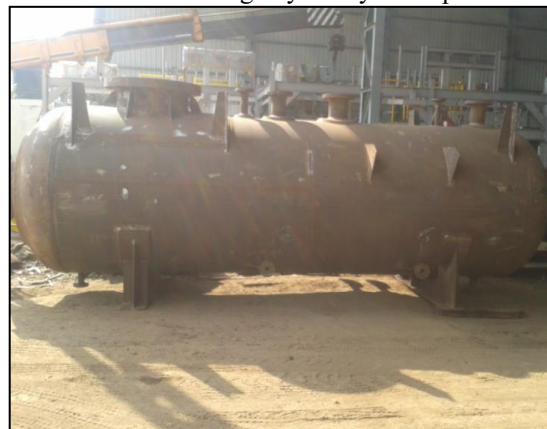
Fig. 1: The typical horizontal storage vessel in fabrication shop
