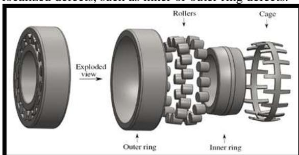
Fig. 1: components of SRB
