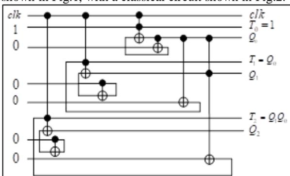
Fig. 1: reversible circuit of MOD-8 counter with TFF
