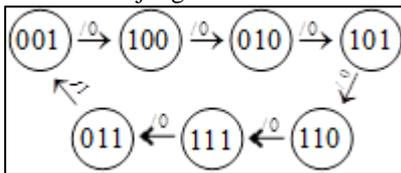
Fig. 3: (a) states transition diagram of MOD-7 counter
