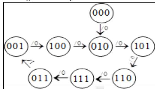
Fig. 4: (a) states transition diagram of MOD-7 counter
