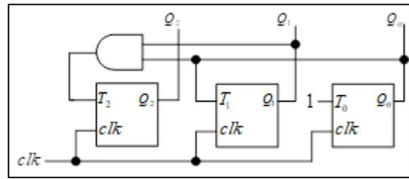
Fig. 2: classical circuit of MOD-8 counter with TFF
