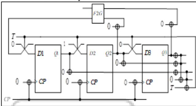
Fig. 5: the design of a MOD-7 self-start counter
