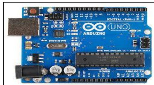
Fig. 3: Arduino Uno board
