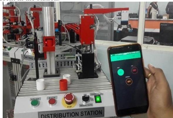
Fig. 8: Distribution station (Mechatronics station)
