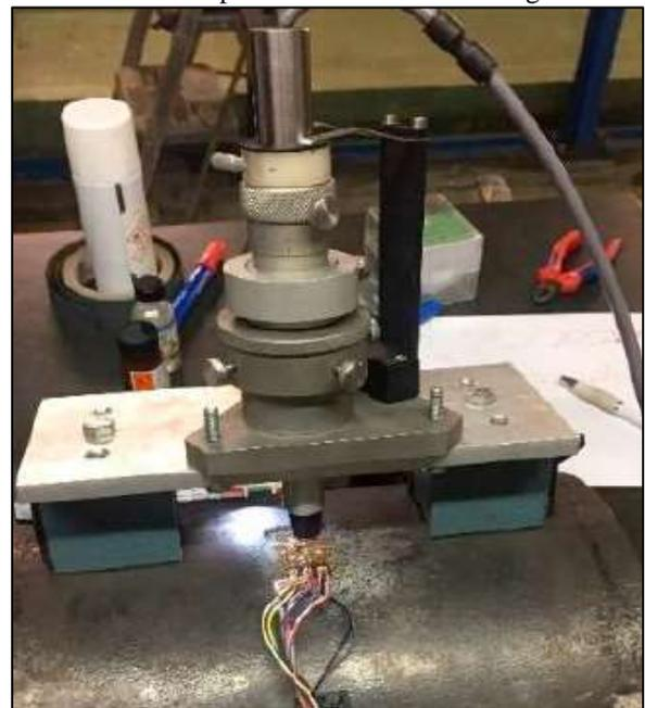
Fig. 5.2: RS200 milling machine
