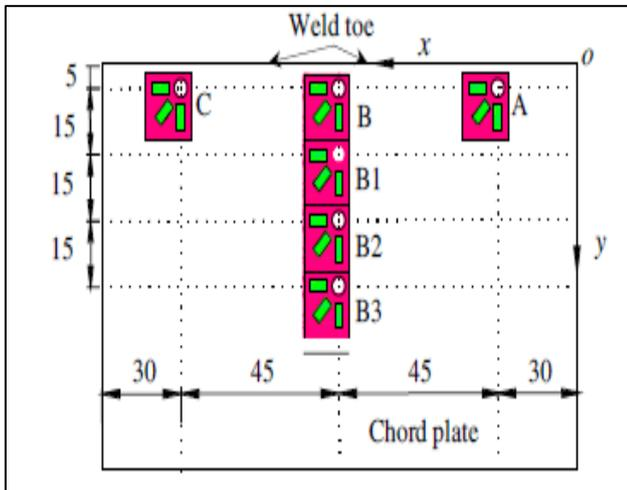
Fig. 5.3: Position of the installed rosettes on the plate
