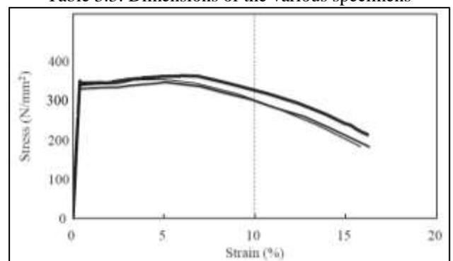
Fig. 3.2: Calculated stress strain curves of S345 steel plates
