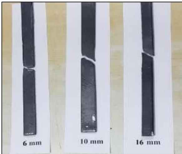
Fig. 3.3: Image of fractured test strips of various thickness
