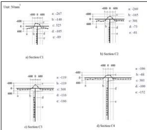
Fig. 6.1: Distribution of the residual stresses at various points
