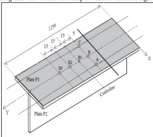
Fig. 5.4: Position of the installed rosettes on the plate
