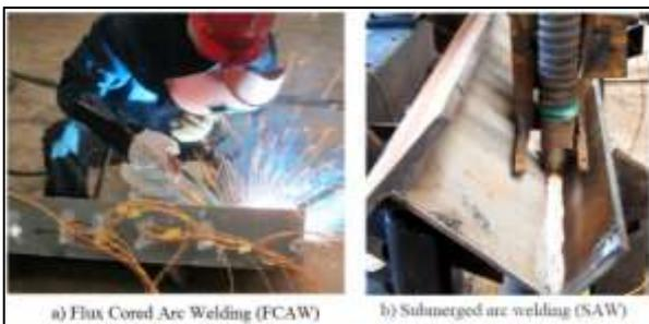
The welding electrodes were in the form of wires. The welding electrodes E71T-1C and EM12K were employed for FCAW and SAW respectively accordance to AWS A5.36<sup>[4]</sup> and AWS A5.17<sup>[3]</sup>. Detailed welding parameters of the two processes are presented in Table3.4.
