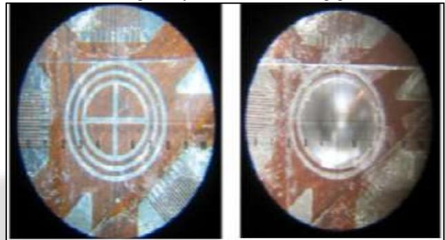
Fig. 5.1: Rosette before and after hole drilling
