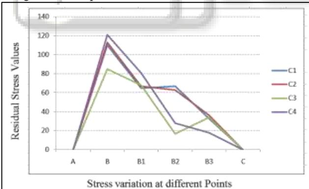
Fig. 6.3: Variation of residual stresses at given points
