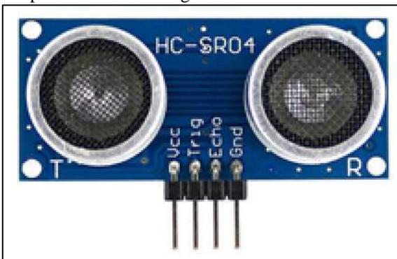
Fig. 2: Ultrasonic Sensor
