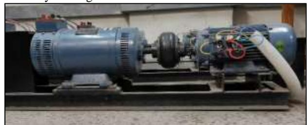
Fig. 3: Motor generator bench arrangement for data acquisition
