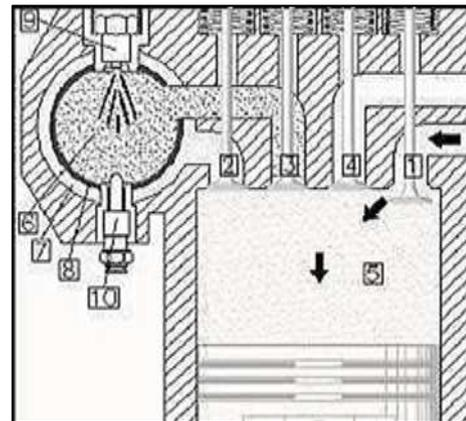
Fig. 1: Components of Six Stroke Engine
