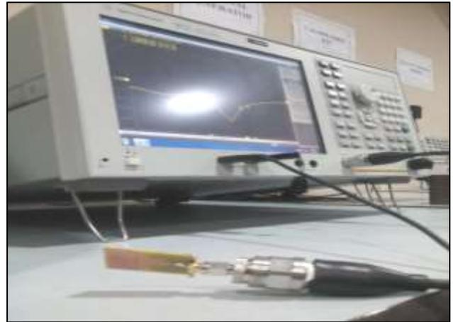
Fig. 3: VNA Testing of Proposed Antenna
