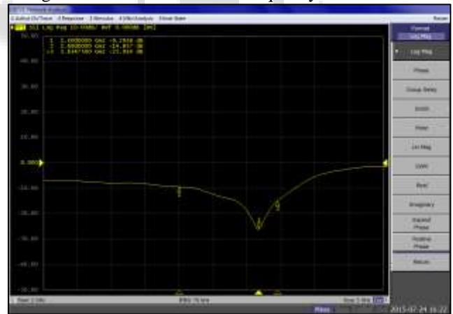
Fig. 6: Measured return loss vs. frequency curve on VNA
