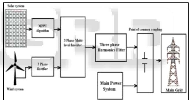
Fig. 1: Block diagram of solar and wind based microgrid
