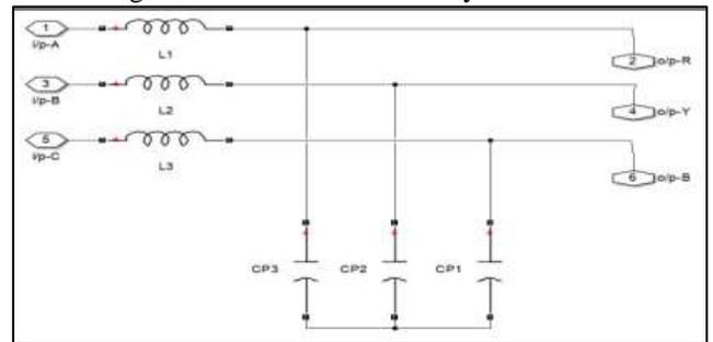
Fig. 6: LC filter for harmonics reduction of inverter output
