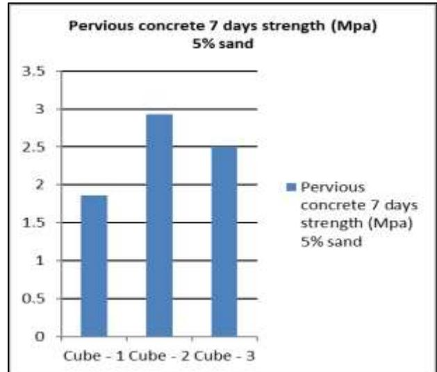
Graph 1: Size of Aggregate 10mm to 12.5mm
