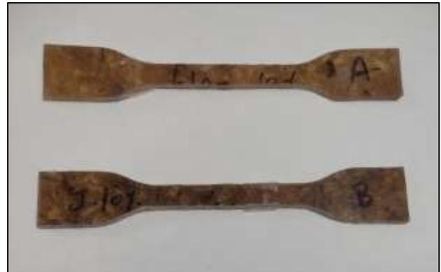
Fig. 2: Tensile test specimen
