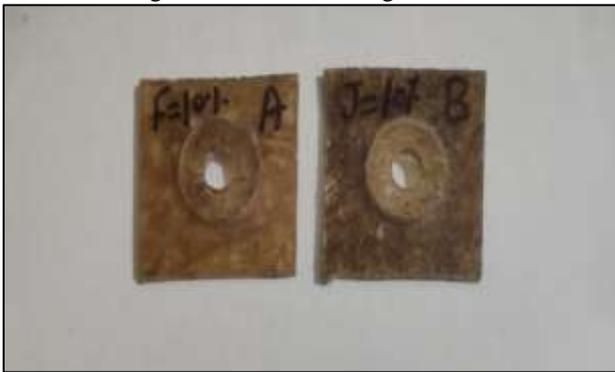
Fig. 6: Shear Test specimen
