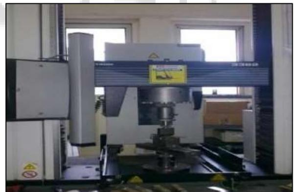
Fig. 3: Universal Testing Machine
