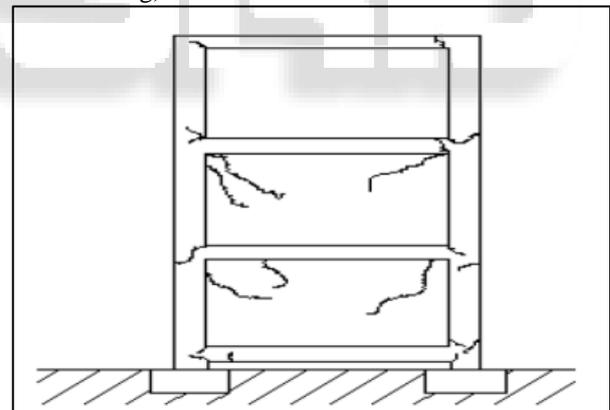
Fig. 2.8: Failure pattern of a fixed based structure due to lateral seismic loading.
