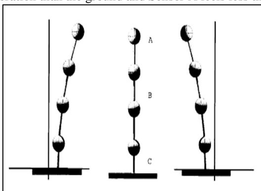
Fig. 1.2: A multiple degree of freedom subjected to ground motion.
