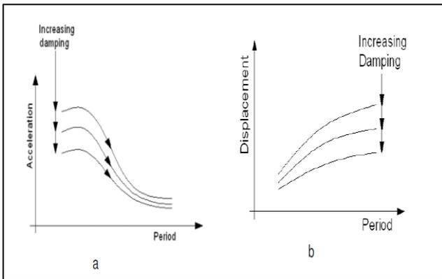
Fig. 2.5: Acceleration and displacement response Spectrum for increasing damping. (a) Acceleration RS, (b) Displacement RS.
