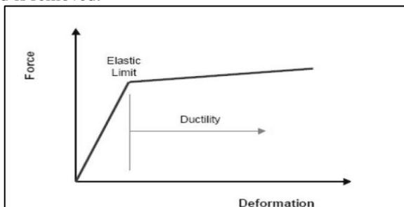
Fig. 2.10: Ductility: deformation beyond elastic limit.
