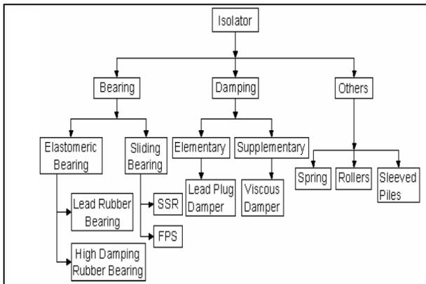
Fig. 2.11: Schematic Diagram showing various types of Isolators used throughout the world.
