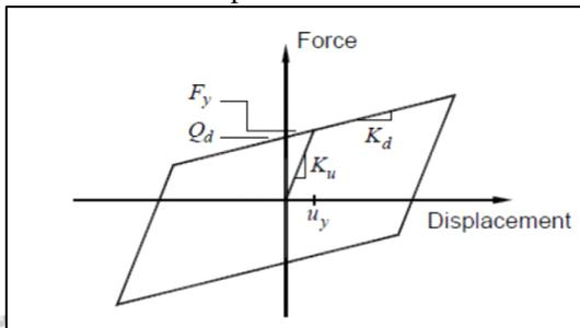
Fig. 2.6: Idealized force-displacement (Hysteresis) Loop.
