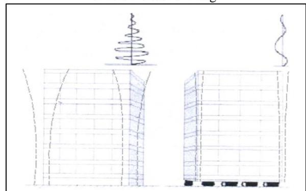
Fig. 2.9: Fixed base and isolated base.
