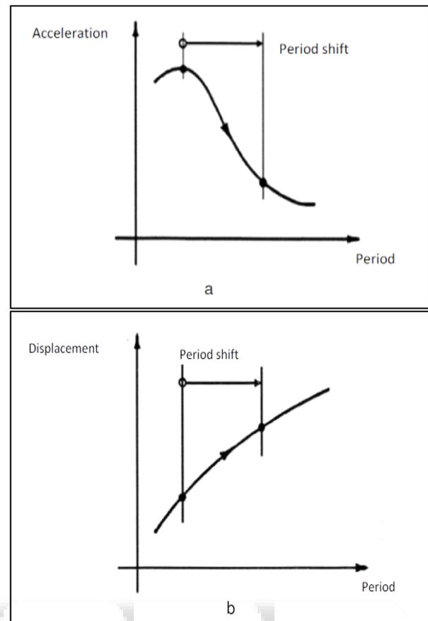
Fig. 2.4: Impact of period elongation obtained by seismic isolation on accelerations. (a) Acceleration response spectrum, (b) displacement response spectrum and displacements of a structure.
