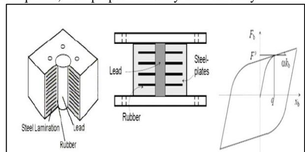
Fig. 2.12: Geometry, schematic diagram and ideal force – deformation behavior of LRB.
