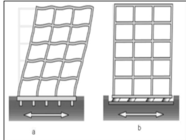
Fig. 2.1: Behavior change while using isolator. (a) Conventional structure (b) base –isolated structure.
