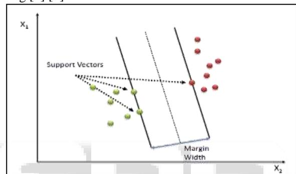
Fig. 4: Working of Support Vector Machine [8]
