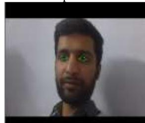
Pic 1: In this pic, our application is detecting the eyes of the driver
