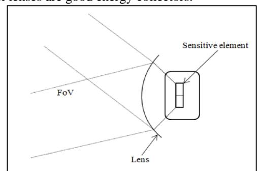
Fig 3: Schematic of typical PIR sensor
