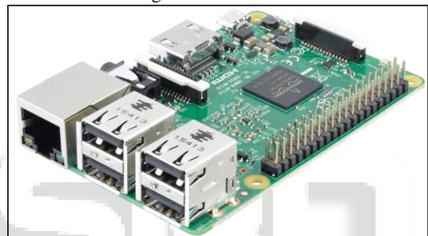
Fig. 2: Raspberry Pi 3 Model B
