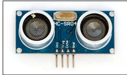
Fig. 5: Ultrasonic sensor
