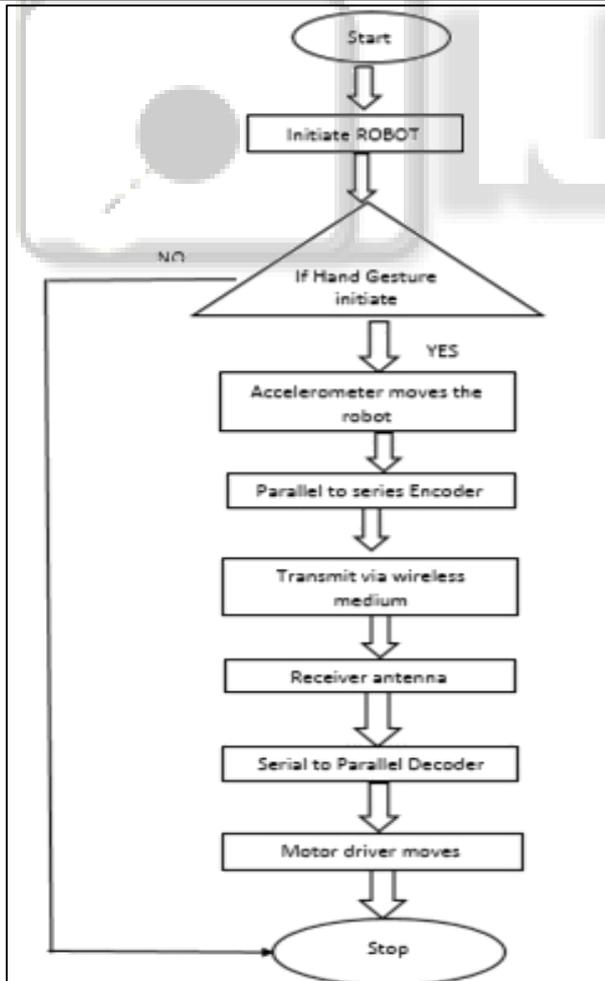
Fig. 7: Dataflow Diagram of GESBOT
