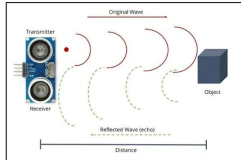
Fig. 6: Ultrasonic sensor working principle
